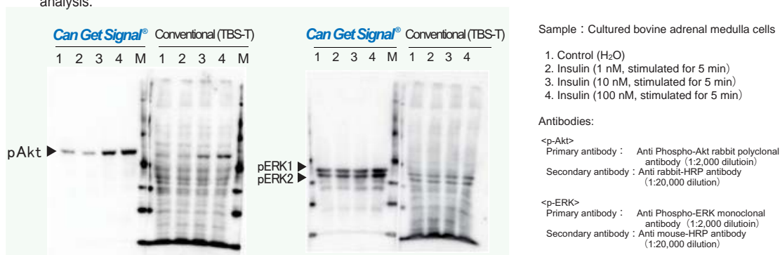
Fig Detection of phosphorylated protein kinases (p-Akt, p-ERK1 and p-ERK2) by Western blotting with Can Get Signal ® and a conventional method
