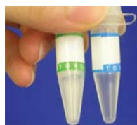
State of the reagents at -20 °C Left: Ligation high Right: Ligation high Ver.2
